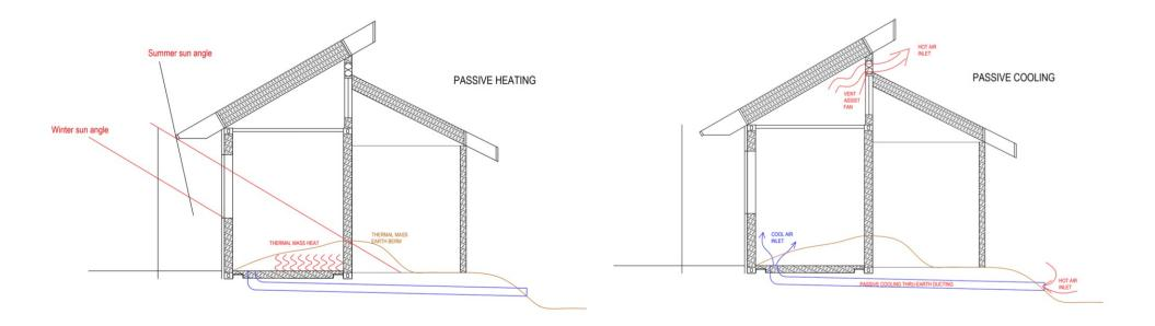
•One of the most significant features of our design the passive heating and cooling. The orientation of the buildings, overhang of the roof and window placement optimizes the heating of the thermal mass of the earth berm during the winter and having shade in the summer. The passive cooling is facilitated by the high ceilings that slope to the north and powered by solar-powered vent fans that draw air through 40' of steel ducting that is buried under the earthen mounds.
